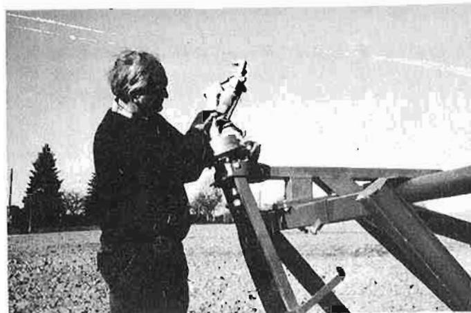
Adjust the part circle setting of the wide-range sprinkler (approx. 220° for full strip width). Refer to sprinkler manual for detailed instructions . Adjust the WIND-GUN to the prevailing wind conditions by changing the trajectory angle.
