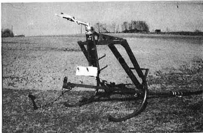
Lower the sled hydraulically and secure it on the ground with the chain and the earth nail.
