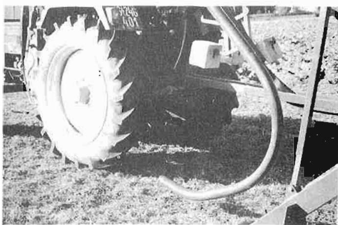
Pull off the PE-pipe (max. driving speed 5 km/h). Avoid sudden stops, slow down gradually in the field or when the pipe has been fully unwound. Stop pulling off the pipe as soon as the white marking on the reel becomes visible.
