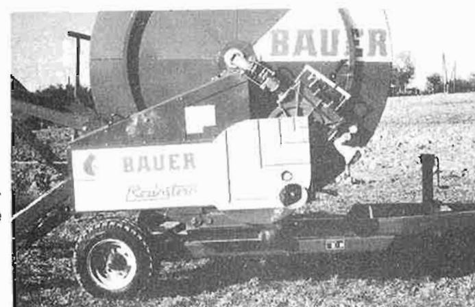
For pulling off the PE-pipe laterally, pull out the lock pin swivel the reel until parallel with the irrigation lane, and secure it again with the lock pin.
