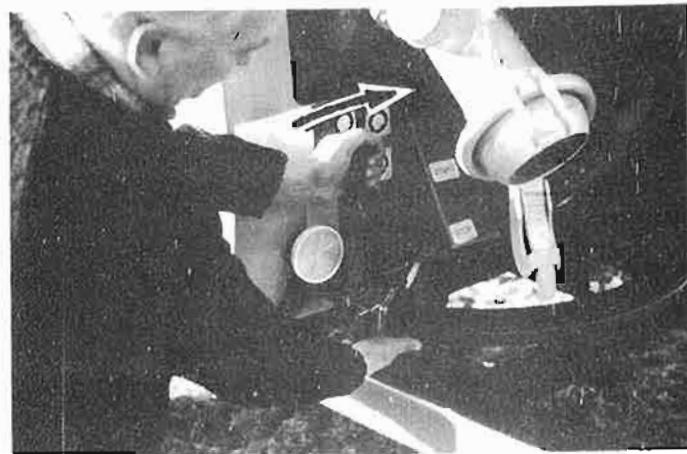
Now disengage the drive by shifting the coupling lever to the "pulling off PE-pipe" position.
