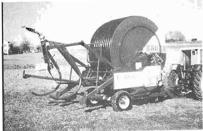
Position the Rainstar on the headland at right angles to the selected irrigation strip and unhitch it from the tractor.
