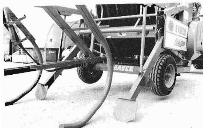
When the supports are extended or retracted the sled is automatically lifted to its transport position or lowered to its working position. The return stop of the drive secures the sled in the raised position (transport position).
